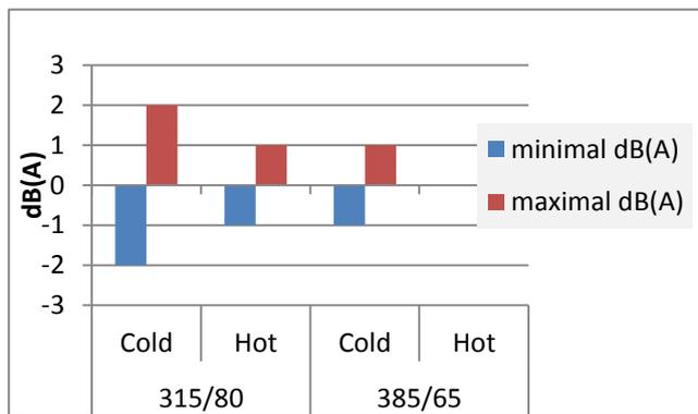
Globally, process parameters can change the sound emission value by 4 dB(A).
