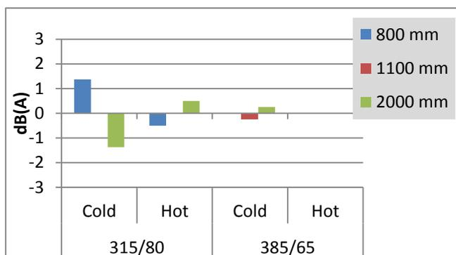
Buffing radius impact is low, but higher for the 315/80R22.5 retreaded with cold process,.
