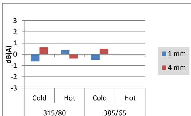
Remaining rubber impact of is low, reaching up to 1.3 dB(A) for the 315/80R22.5 hot retread, but lower for other configuration
