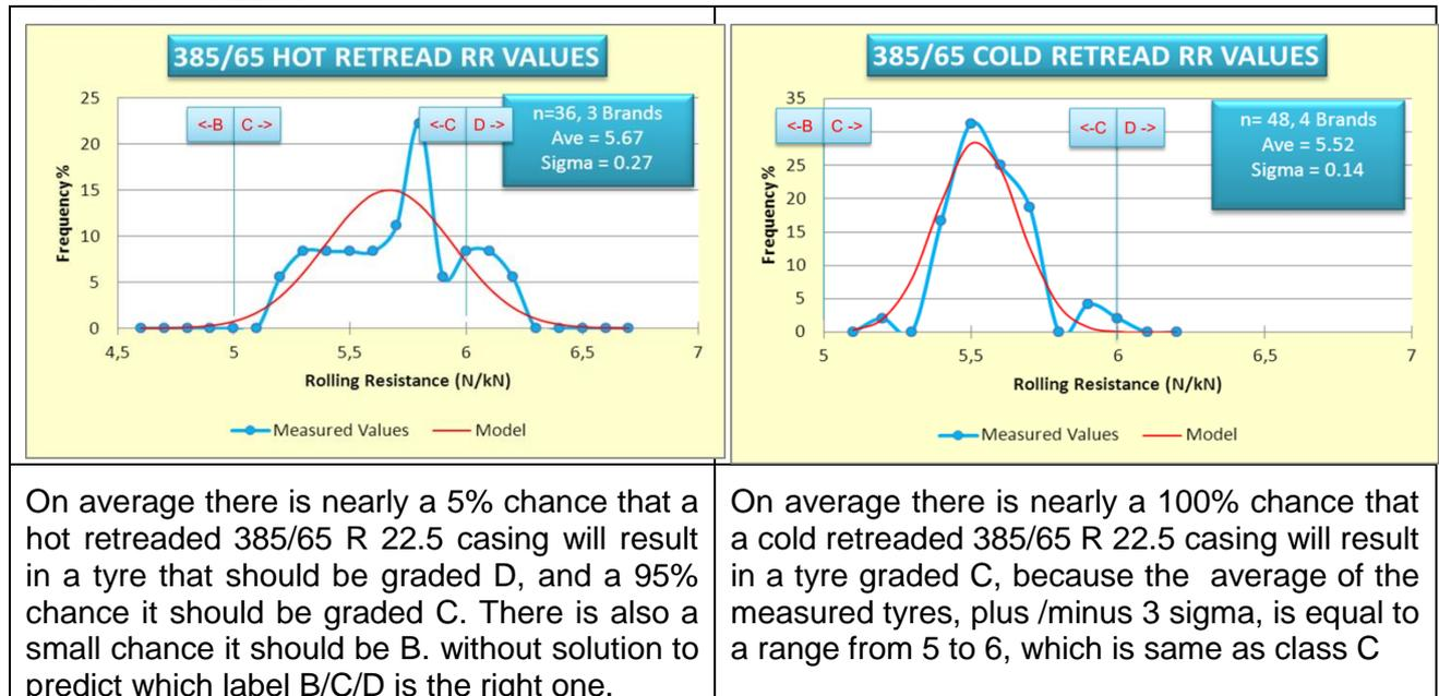
Data show that rolling resistance of retreaded tyres sample are spread on at least 0.73 N/kN (385/65 Cold), and up to 1.23 N/kN (315/80R22.5 Cold), not including spreading of population assuming a Gauss repartition, which would increase the spread up to 1.74 N/kN with 6 sigma. Depending on the average value, these values indicate that at least 2 labels will be covered by one
