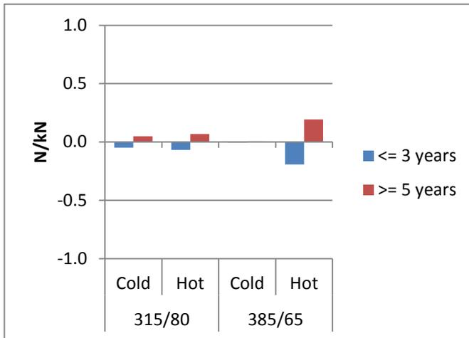
Comparing the average of each casing brand to the central value, these data show that casing age (lower or equal to 3 years, or superior or equal to 5 years), A slight trend of rolling resistance increasing with casing age can be observed, especially for 385/65R22.5 with hot retread. However, the possible impact seems low, and should be confirmed by an extensive survey.
