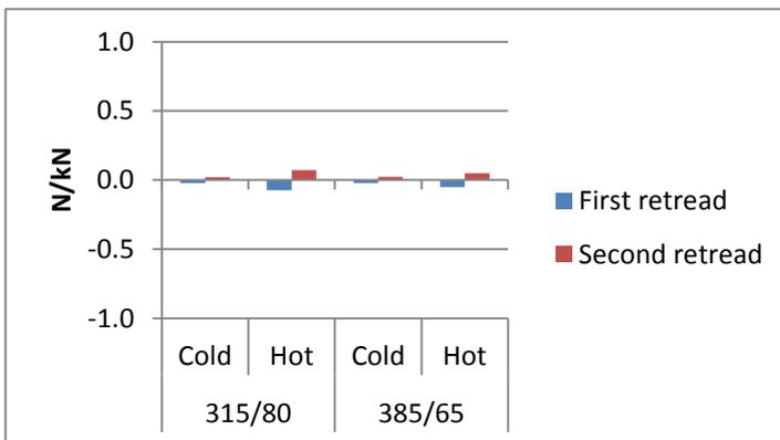
No significant impact can be observed for cold retread. However, for hot retread, a trend to increase of rolling resistance with number of retread can be observed. To be confirmed.
