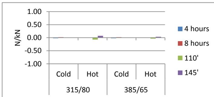
Impact of curing temperature is high for hot retread, whatever is the size, and lower for cold retread
