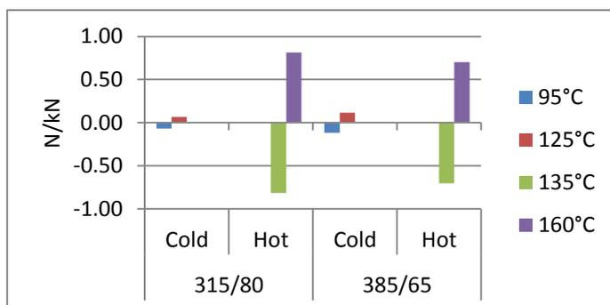
Impact of curing temperature is high for hot retread, whatever is the size, and lower for cold retread
