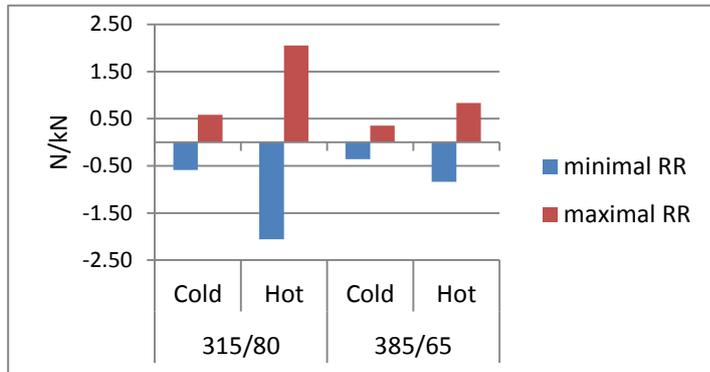
Globally, process parameters can change the rolling resistance value by up to 4 N/kN, which represents 4 labels.
