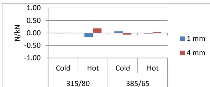
Impact of remaining rubber is low, reaching up to 0.35 N/kN for the 315/80R22.5 hot retread, but lower for other configuration
