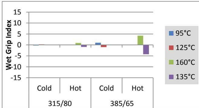
Curing temperature impact is very low, but for 385/65R22.5 with hot process, where impact is low
