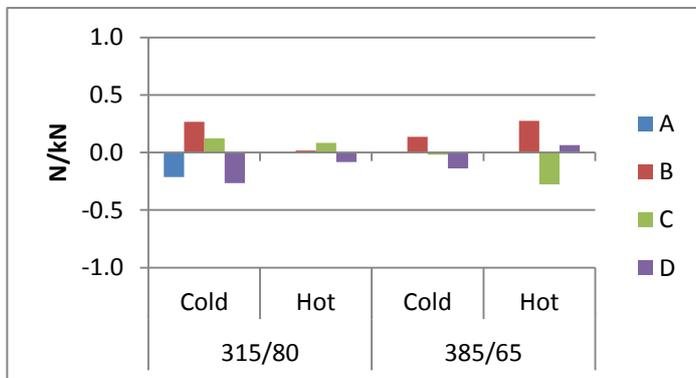
Comparing the average of each casing brand to the central value, these data show that casing brand has a strong impact on the final result (range up to 0.55 N/kN)
